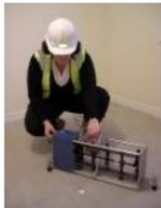
Figure 4 Impact sound test being carried out
