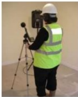
Figure 1 Sound test being carried out
